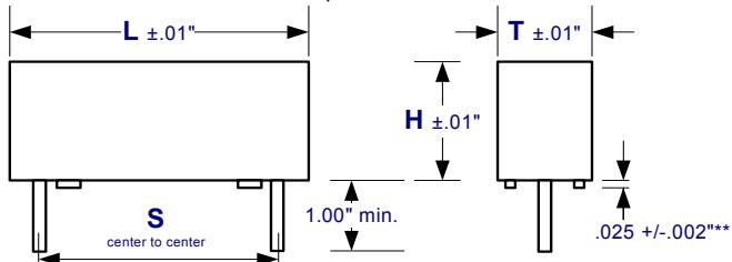
\*\* Mounting pads consist of two individual pads on each end or one continuous pad on each end, depending on the mold.
